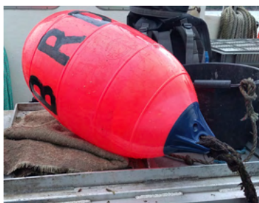
▲ The use of low-drag buoys will be investigated during further trials, to see how effective these are at reducing the risks of the tide and swell dragging gear over the seabed.
