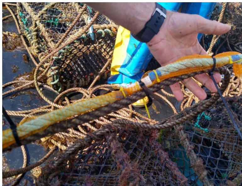
▲ Sensors were mounted on the ropes, to record how they moved during the tidal cycle when the gear was on the ground.
