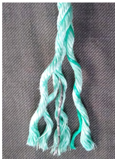
▲ The sinking rope has a thin core that runs through the weave. It is available in all of the normal diameters – but the cost is significantly higher, so widespread take-up would depend on funding support.
