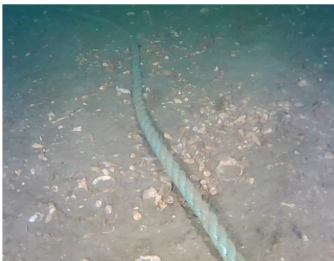
Figure 5.9. A still from ROV footage showing sinking groundline which has been lying on seabed for 10 days
